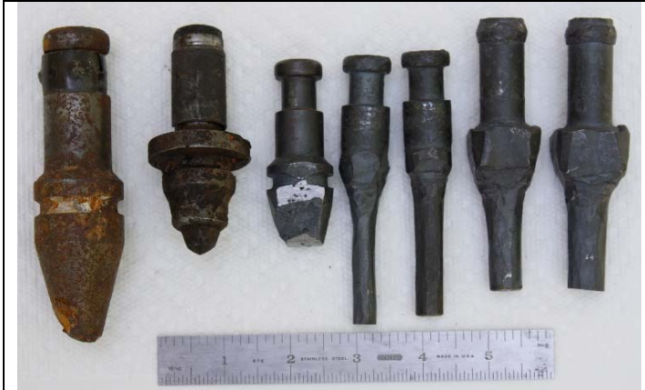
Fig. 1. Raw road milling bits on the left and partially finished tools on the right.
