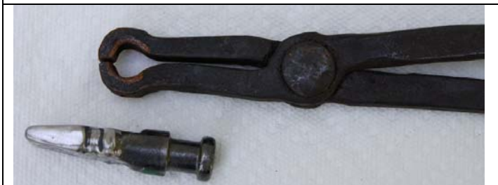
Fig. 4. Tong re-made to hold tooling.
