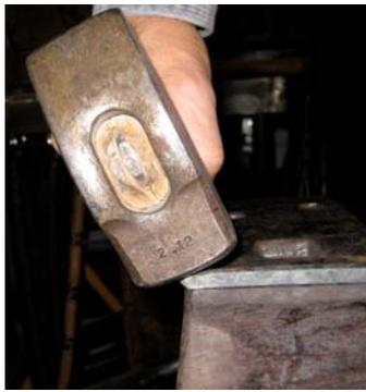
In the drawing out process you will make ripples in the metal formed by the edge of the hammer on top or by the edge of the anvil on the bottom. After you have moved enough metal to form the taper, place the
