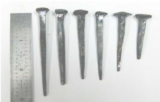
decided to use a cold-cut Hardy tool and cut the nails cold rather than taking an extra heat and using a hot-cut. These changes greatly speeded up my nail making.
