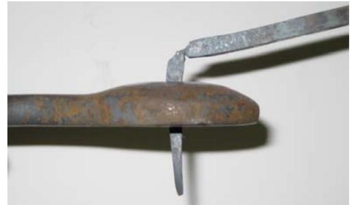
twisting motion. Place the header with nail on the anvil over the Hardy hole and make the head of the nail. The first few hammer blows should be directed
