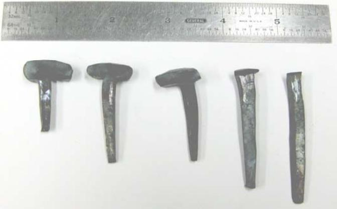
On the second rainy day, Friday, I made a square punch and opened up the bottom of the square hole in the nail header a little bit. This allowed the header to release the nails cleanly without much more than a gentle tap and without quenching. I also
