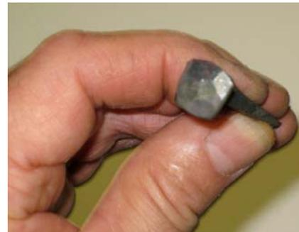
to make the metal centered on the stem of the nail. This may require some angled blows. Once the metal is centered it should take about five
