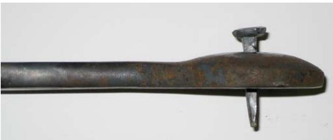
At this point you have completed a cycle. One iron is tapered, partially cut but cold, and the other iron is raw but hot and ready to be headed. *More importantly, there is a completed nail on the floor.*
