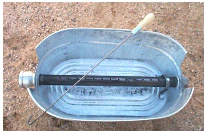
The tuyere is 1" ID black pipe(not galvanized) and is 18 inches in length. It can be cut and threaded on both ends for free there when you buy the pipe. The oval tub is also available at Home Depot too but they seem to run out often and restock slowly. I used the 3.75 gallon size in the video but the larger
