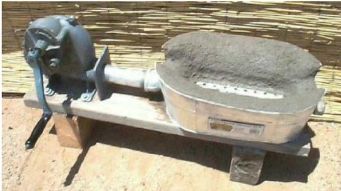
Here's the forge with the adobe in it and connected to a hand crank blower. It will need to sit until bone dry before its first fire. You have to provide the air supply as in blower, bellows or hair dryer etc. and the adobe filler. An excellent adobe for use as filler is made from 1/2 earthen clay and 1/2 sand with a couple handfuls of wood ashes added in.
