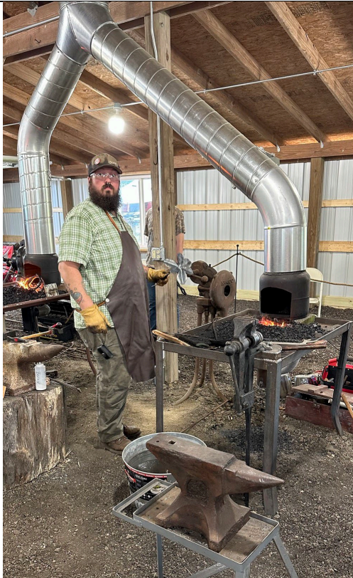
Forge table with coal, side-draft hood, blower, anvil on stand, post vice, water bucket, and blacksmith. Note the large sheet metal stovepipe to remove smoke.
