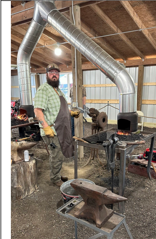
Forge table with coal, side-draft hood, blower, anvil on stand, post vice, water bucket, and blacksmith. Note the large sheet metal stovepipe to remove smoke.
