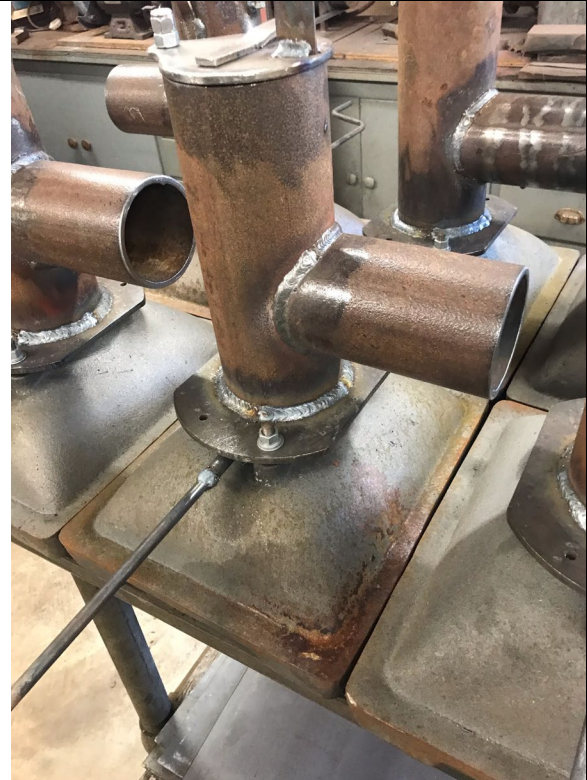
Underside of the fire pot showing the ash dump and air pipe. We have 11 of these.
