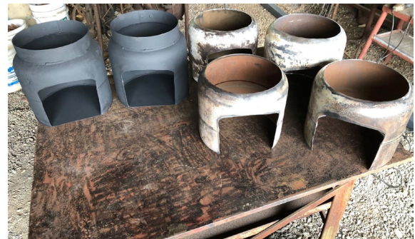
Super-suckers in various stages of completion made from propane tanks.
