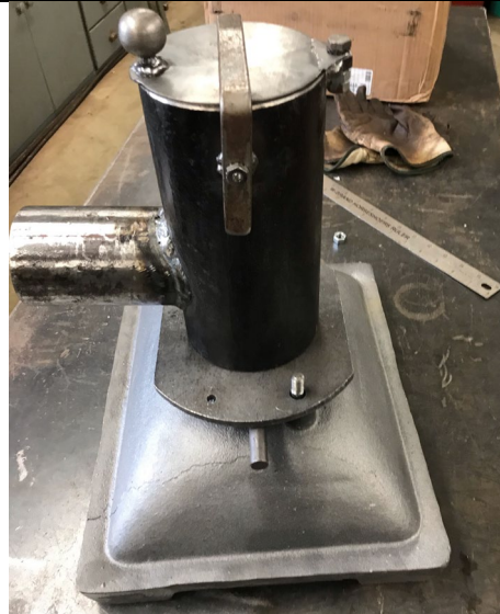
New coal forge fire pots that we bought, and the ash dumps we added.
