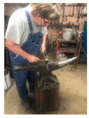
This will help to keep your fingers from burning as you are using the tongs with gas forge. After you have your marks on where the fullers will go it is best to use the anvil to mark it cold. This cold mark will allos you to find it when the piece is hot. Next comes putting the fuller marks in the piece. The fullers will need to be half the thinkness of the stock. This is accomplished by using bar fuller as shown in the picture. Fuller down until stock meets the anvil. As you move the
