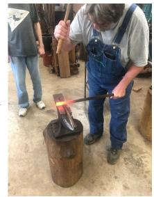
begins the real work. Draw out the 7 inches of rein stock to 14 inchs. At the end of the first rein I started I wished I knew how to forge weld.
