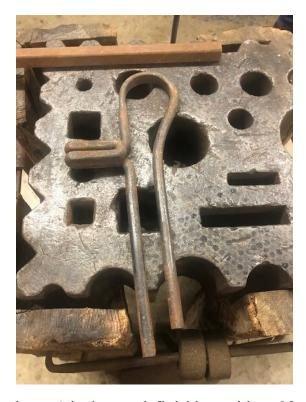
about 6 inches and finishing with a 90 degree turn. Heating and bending over the doubled section forms a square area that can be used for the Hardy. All that is left is to put a bend in the rod forming the spring. See the picture for a dimentional view. The cutoff tool is very similar but instead of leaving a rouned rod to make them into triangles with the points towards each other.
