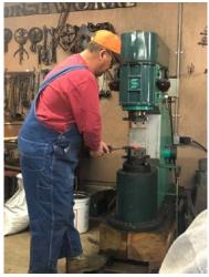
lighter to use. Of course, like any good teacher Kurt reinforced the blacksmith mantra with us to always work our metal square, octogan, round. In the two power hammer pictures Kurt is first working by self and then Craig helping in a later step to create a step tool for making the jaws of the tongs. The step tool assists in making a pair of tongs without having to twist the jaw. The reasoning behind this is to avoid the twist to help make the tong jaws stronger.
