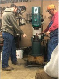
between a punch and a drift so I asked. Kurt explained that a punch is designed to punch a hole where a drift is designed to widen a hole. He also recommend to make them slightly larger to allow for the shrink.
