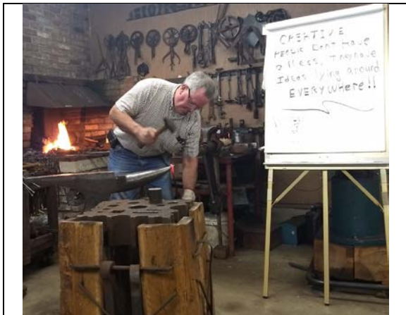
Gary shows how to widen the bottle opener hole without thinning the material too much.
