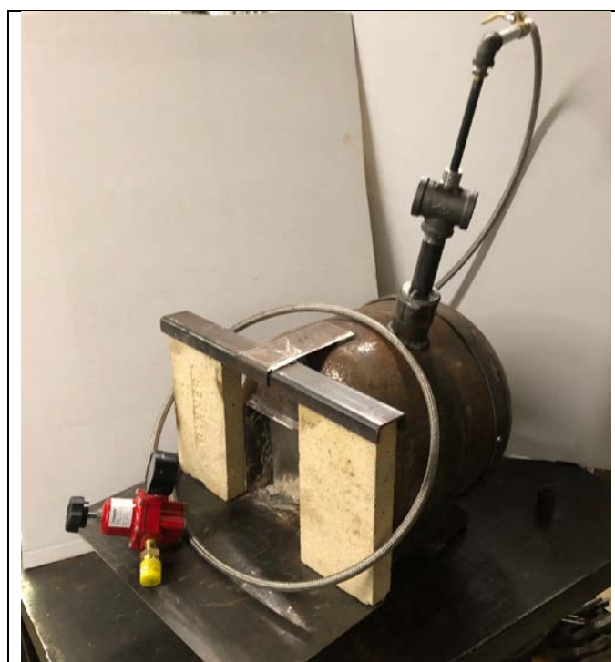
One of the 25 completed propane-powered gas forges made by and for the Rocky Forge Blacksmith Guild.
