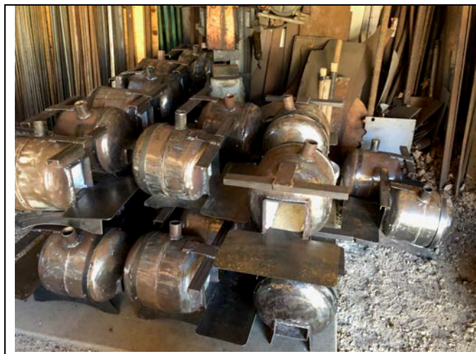
These 22 gas forges are insulated and are awaiting the installation of the burner, hose and regulator. Some of these may be ready for distribution at the October 9 th meeting.
