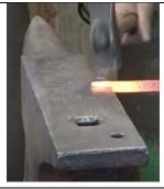
Draw out the ring metal and get graceful taper and make the metal have a round cross section.
