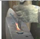
Split the tines from top and bottom with a chisel starting with light blows. Use soft metal under piece to protect.
