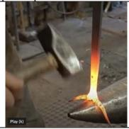
Make tines have round cross section. Shape tines on the horn to the desired distance apart.
