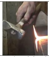
Square up tines on the face and on the side of the anvil. No need to eliminate the v-grove.
