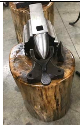
Jim Claar anvil with integrated swage block.
