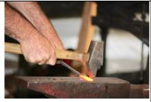
Here Mark is forging the part of the tong jaws that will hold the workpiece from the side. First, he isolates the material, and then he pushes it out. The final step involves lifting the material to form the side of the tong jaw, i.e. the part that keeps the workpiece from sliding around in the jaw.
