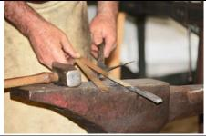
Mark is using a 24-inch folding brass farrier's ruler to measure an important dimension his workpiece. These rulers can be purchased at most farrier supply shops such as <a href="http://www.americanfarrierssupply.com/m5/760--fpd-folding-brass-ruler.html">http://www.americanfarrierssupply.com/m5/760--fpd-folding-brass-ruler.html</a>
