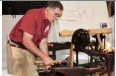
Mark forging a set of tongs. Notice that Mark is right handed and sets the heel of the anvil in front of his right hand. Many, but not all, smiths prefer this arrangement. He is also wearing eye protection and a leather apron. Mark prefers to smith without gloves on either hand. Some smiths wear a glove on their non-hammer hand because that hand gets beat up from holding the workpiece or tongs.
