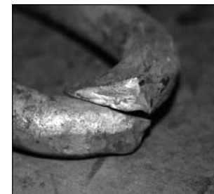
Fig. 5. Weld on the anvil face first. Work quickly and from both sides of the link
