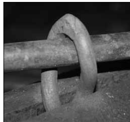
Fig. 8. Test your weld by twisting it and then straightening it out again
