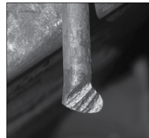
Fig. 3. Rotate the stock as you hammer to draw the scarf
