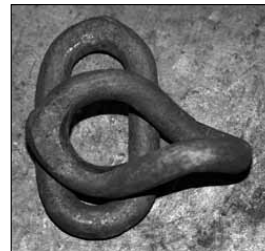
Fig. 9. A chain link in the midst of testing
