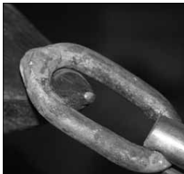
Fig. 7. Rotate the link back and forth around the horn
