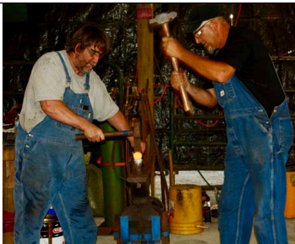
John Bennett and 2018 IBA Blacksmith of the Year, Steve King, make a rose from a 2" thick steel cylinder.
