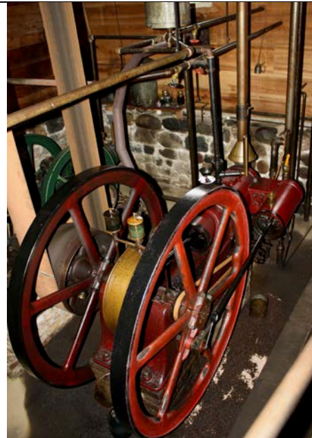
Shop is mechanically powered by this hit-and-miss engine and a complicated series of line shafts.
