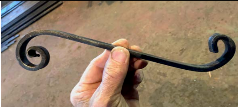
Kurt made a teaching piece showing good scroll on the left and bad scroll on the right.
