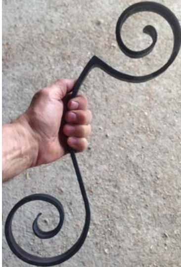
The right angle is made using angle iron that is forge welded into this piece.
