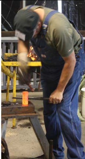
Steve King forges face of hammer head.
