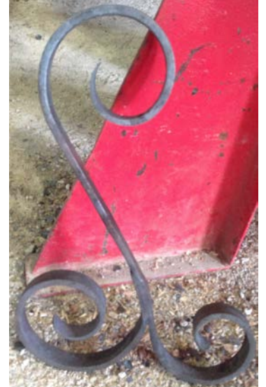
Basic scroll shape made using two forge welds.
