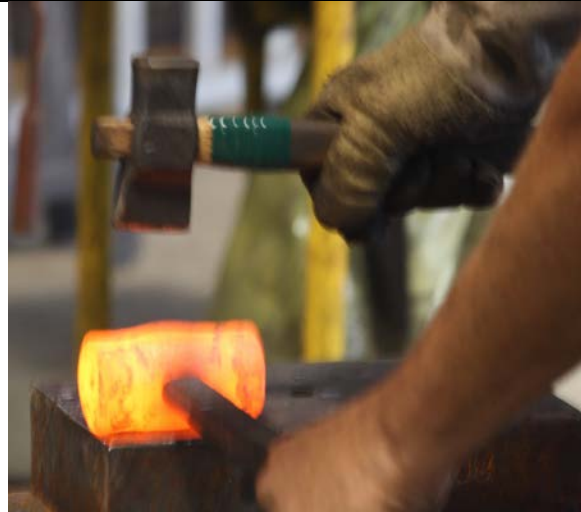
Steve King uses a fuller to shape the head. A striker on the left will hit the fuller.
