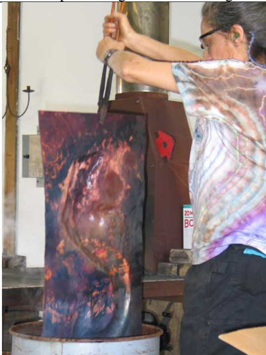
Annealing after heating with a propane weed burner.
