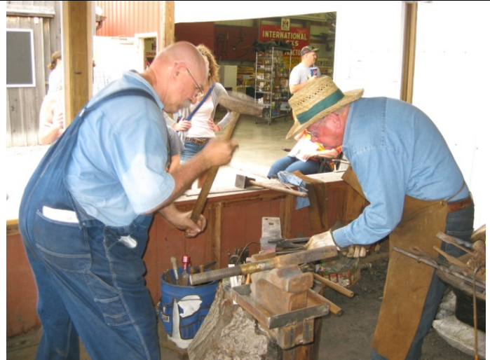
Bill Newman and Ted make an ax. Bill provides the horsepower and Ted the finesse.
