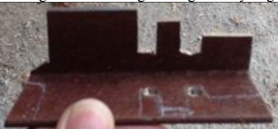
Close-up of the symmetrical pattern cut from angle iron. Only one side is cut away.
