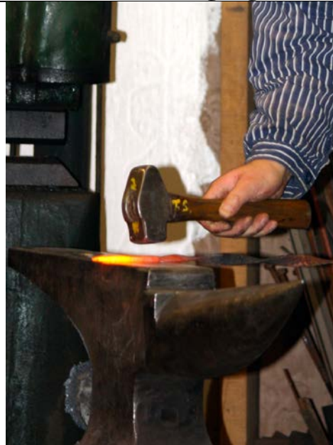
After welding, get primary shape.
