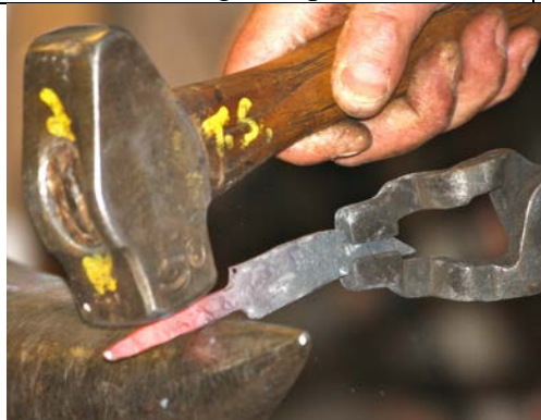
Draw out the tang on the anvil horn.
