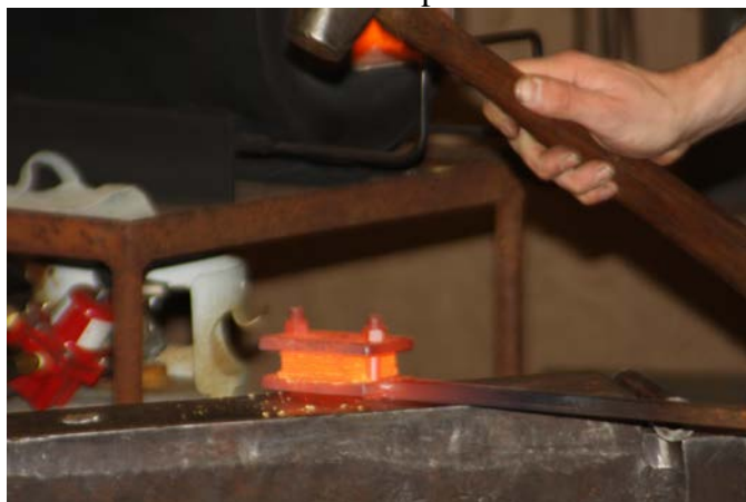
30 layers of copper and brass being forge welded in a special holder. The layered ingot can then be shaped in various ways to get a desired final pattern.
