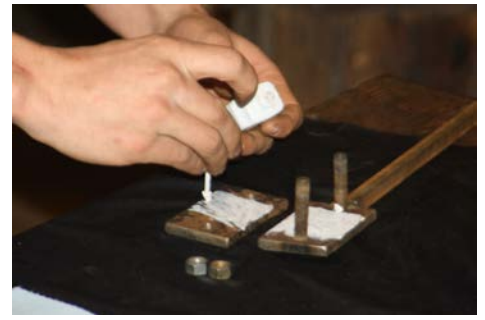
Snopake helps release welded metals.
