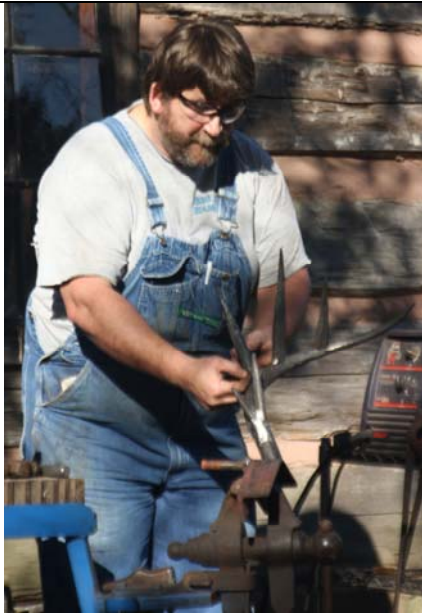
Weld on the spokes and fill-in and grind the joints.
