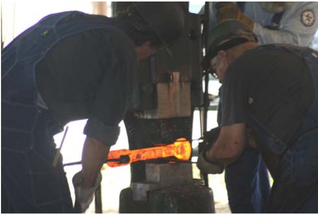
Steve Parker and Clifton Ralph examine the vice jaw under the two hundred pound Chambersburg steam-driven power hammer.
