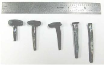
On the second rainy day, Friday, I made a square punch and opened up the bottom of the square hole in the nail header a little bit. This allowed the header to release the nails cleanly without much more than a gentle tap and without quenching. I also
