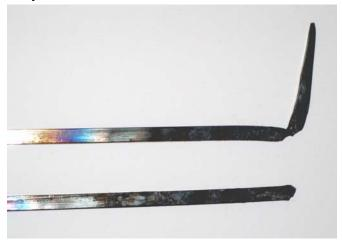
**Step 1 (Taper and cut):** Remove the hot raw iron from the fire. Taper and partially cut the raw iron and return it to the fire. At this point you have two tapered and partially cut irons in the fire.
