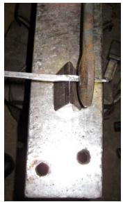
cut at the measured location. Cold cut most of the way through the stock. Rotate the stock as you cold
