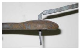
twisting motion. Place the header with nail on the anvil over the Hardy hole and make the head of the nail. The first few hammer blows should be directed
