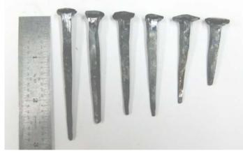
decided to use a cold-cut Hardy tool and cut the nails cold rather then taking an extra heat and using a hot-cut. These changes greatly speeded up my nail making.
