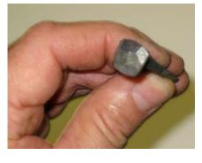
make the metal centered on the stem of the nail. This require may some angled blows. Once the metal is centered it should take about five
