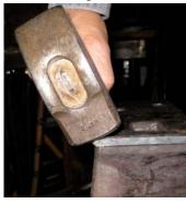
In the drawing out process you will make ripples in the metal formed by the edge of the hammer on top or by the edge of the anvil on the bottom. After you have moved enough metal to form the taper, place the
