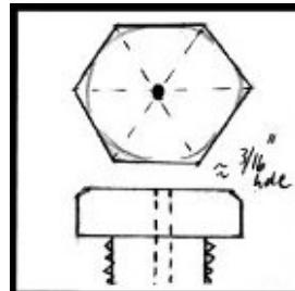
Find the center of the bolt. I scribe lines so they intersect. Then drill a 3/16 hole thru it.
