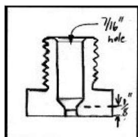
Now flip the bolt over and drill a 7/16 hole from the bottom. But DO NOT go all the way thru. Stop about 1/8 from the edge
