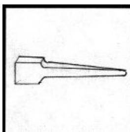
Now the only hard part is to draw the bar down till it is a comfy fit to the hand. Mine ended up about 10 in long. If you have a pwr hammer no problem, but I did it with a 2.5 lb hammer.
