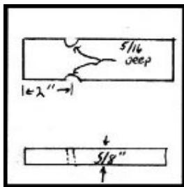
Two inches from one end fuller the edges. I go about 3/8 in deep and use a fuller that is made from 3/8 round rod.
