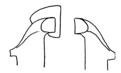
Bring to welding heat with steel up in fire.
