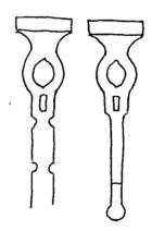
Draw material between fullers to a taper from over 1/2" to under.
