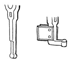
Drill and rivet to vise leg 3/4" above or even with bottom bend depending on space available.
