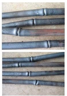
Cut and paste the links into your browser to see them. The bronze version and the first steel version are made with forging and then welding. The third is all forging. I like the forged version best for the steel. For the bronze, I still like the other method.
