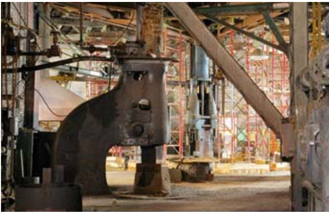
A 4,000-pound Bement-Miles Steam Hammer, ca. 1888. A 3,000-pound Chambersburg Steam Hammer is visible in the background.
