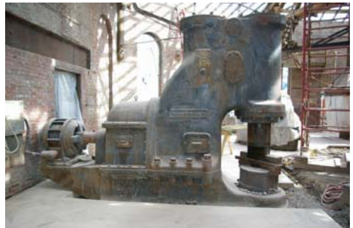
This May 2007 photo shows a new concrete pad that has been poured around one of the shop's hammers.
