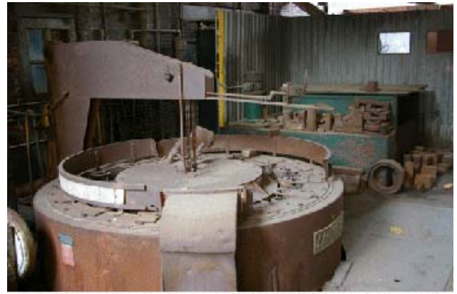
Second Lindberg Pit Furnace. Note steam hammer tooling stacked on quench tank.
