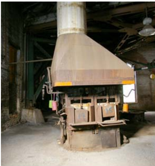
One of several side-by-side gas forges. Each side is an independent furnace, with counterweighted doors front and rear to allow long work to be passed through.
