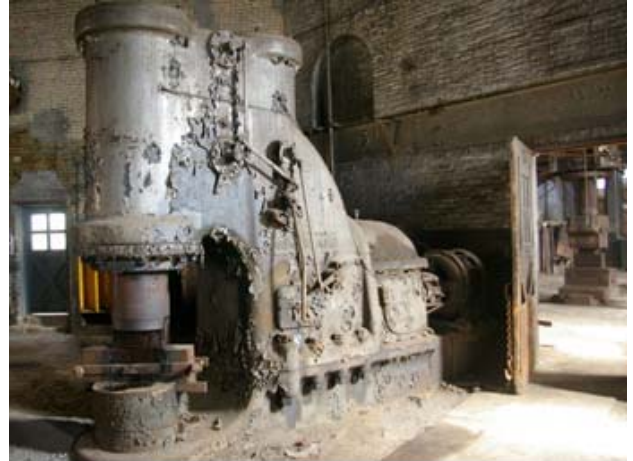
2,000-pound Chambersburg Self-Contained Hammer, ca. 1940, powered by a rear-mounted 75-horsepower General Electric motor.
