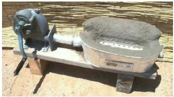
Here's the forge with the adobe in it and connected to a hand crank blower. It will need to sit until bone dry before its first fire. You have to provide the air supply as in blower, bellows or hair dryer etc. and the adobe filler. An excellent adobe for use as filler is made from 1/2 earthen clay and 1/2 sand with a couple handfulls of wood ashes added in.
