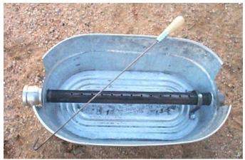
The tuyere is 1" ID black pipe(not galvanized) and is 18 inches in length. It can be cut and threaded on both ends for free there when you buy the pipe. The oval tub is also available at Home Depot too but they seem to run out often and restock slowly. I used the 3.75 gallon size in the video but the larger
