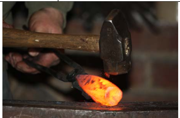
Finish shaping hammerhead, peen and eye.
