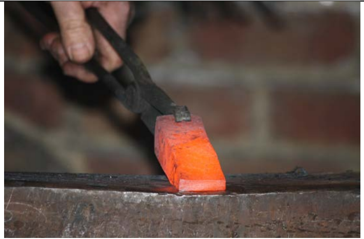
Rough shape of the hammerhead.
