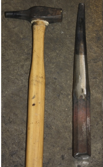
Punch to start hole. Drift to open hole.
