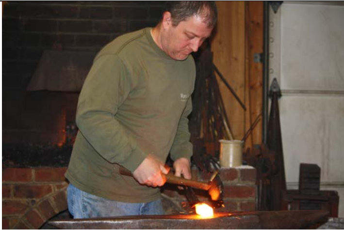
Forge the rough shape of the straight peen hammer.
