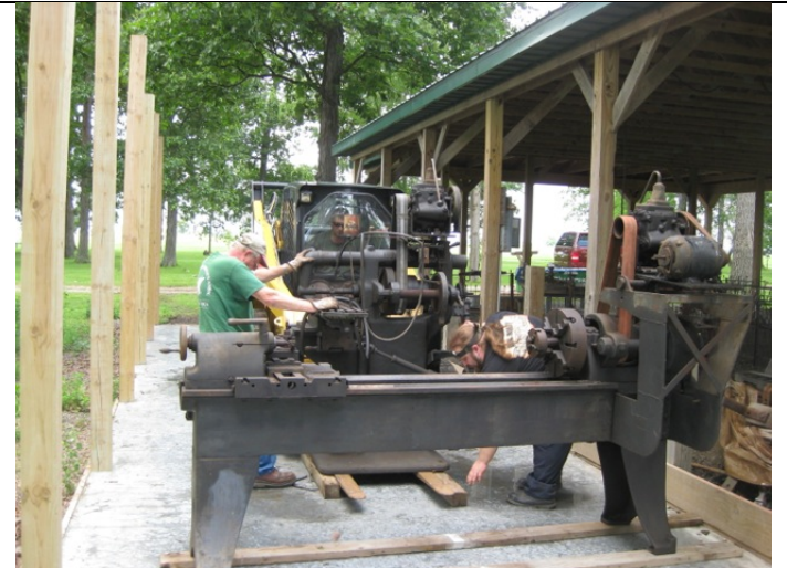
Cory positions wooden block under the shaper as Ted steadies the heavy load.
