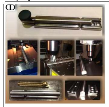
This sliding door latch was made by Dominick using some stainless pump shaft that Gene Hollingsworth provided. Dominick's new mill had no trouble milling this tough material.
