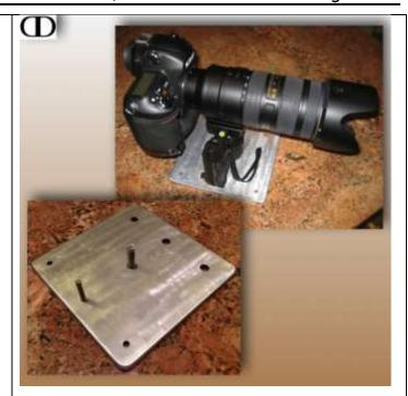
A remotely placed and triggered camera can be mounted on the small platform Dominick milled recently. Aluminum cut like butter compared to the harder stainless steel of his previous project.
